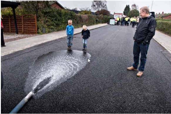
Figure 48: Example of permeable surfacing on Agerlandsvej in Odense ( www.fyens.dk )
