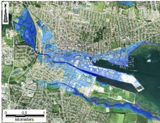
Figure 26: Consequence map for flooding with preliminary outlined proposal that will protect Horsens town in the short term?, equivalent to flood-proofing at a level of 1,8 meter DVR90. The flood proofing will be established using a high tide wall earth dykes and mobile water tubes.
