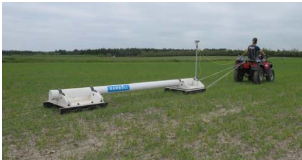
Figure 50: Example of geophysical mapping using DualEM.
