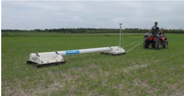
Figure 50: Example of geophysical mapping using DualEM.
