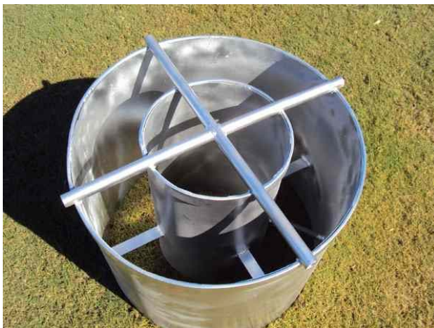
Figure 52: Example of a double ring infiltration test gauge. ( www.turf-tec.com )
