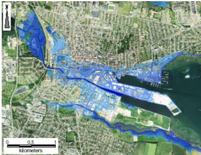
Figure 26: Consequence map for flooding with preliminary outlined proposal that will protect Horsens town in the short term?, equivalent to flood-proofing at a level of 1,8 meter DVR90. The flood proofing will be established using a high tid wall earth dykes and mobile water tubes.
