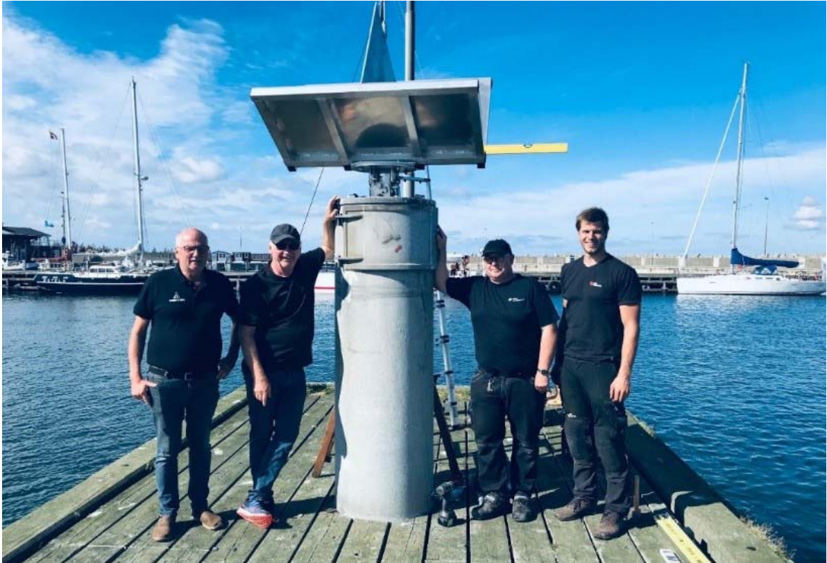
Radar Reflector to measure seawater level at a Danish Harbour
