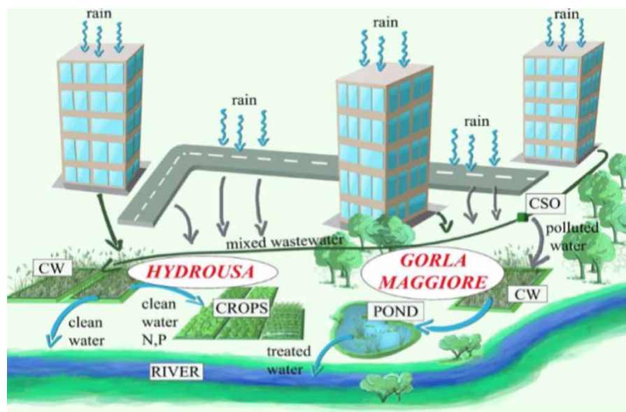
Figure 6 | Transition scheme towards a decentralised and integrated, sustainable water management in an urban settlement with the contributions of the case studies HYDROUSA and GORLA MAGGIORE highlighted (SUDS: sustainable drainage systems, CW: constructed wetlands) (adapted from Masi et al. 2018).
